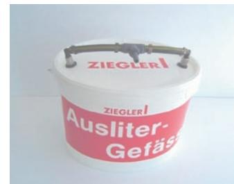
Gauging vessel for buffered acid products (e.g. Lupro-Grain®)
