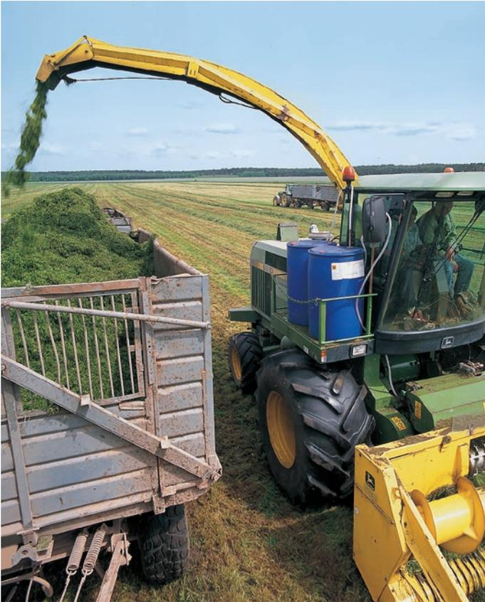
Injection of liquid silage additives
