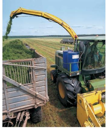
Injection of liquid silage additives
